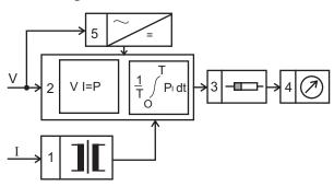
The power converter uses one, two or three multiplier systems 2 depending on the measurement of balanced or unbalanced load AC systems. Current transformers 1 provide the input current to the multiplier circuit.
